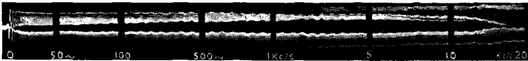
FIG. 17/3.—Response oscillogram of nameless faulty amplifier. Effects of motor-boating, HF oscillations and harmonic distortion are included. Amplifier as used in Figs. 5/2, 5/3 and 5/5.
